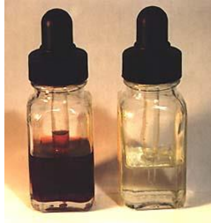
Fig. 2: VP reagents Left is reagent A (alpha-naphthol) and Right is reagent B (KOH--potassium hydroxide)
